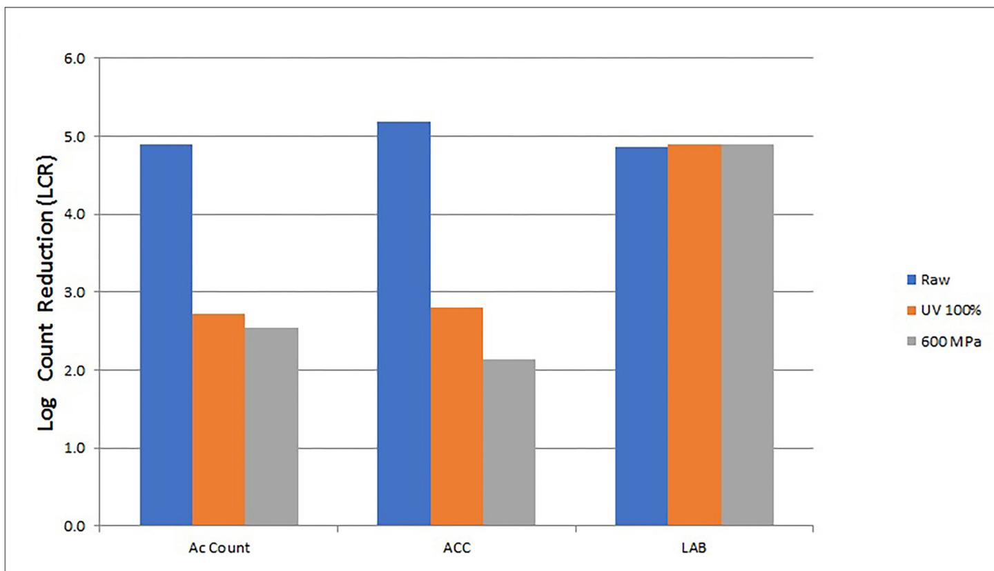
**Figure 3.** The efficacy of the AseptoRay UV system compared to HPP treatment for LCR of natural microflors in a green blend juice
